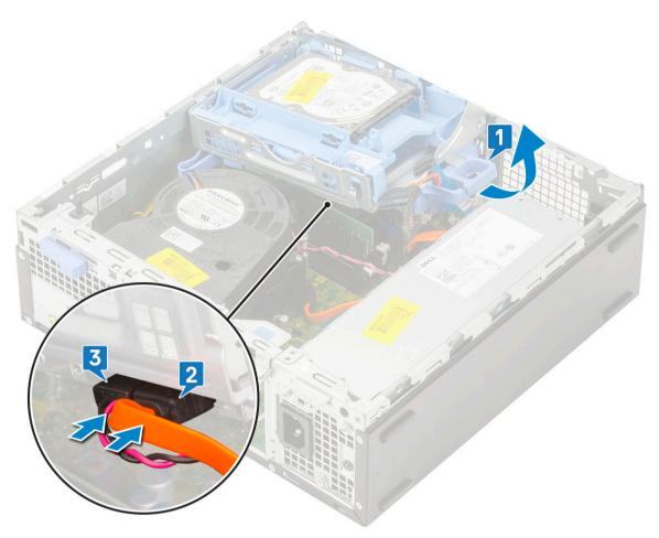
Connect the hard drive data cable and hard drive power cable to the connectors on the hard drive [1,2].
