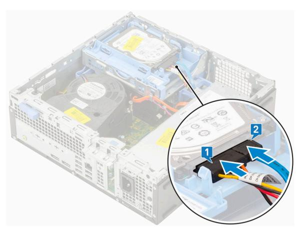
5 Slide the release tab to lock the module [2].
