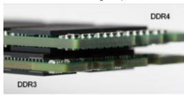
Figure 2. Thickness difference
