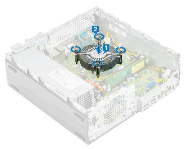
3 Place the heat sink cover onto the heat sink.
