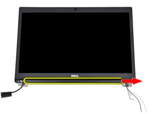
4 Remove the display hinge cap.
