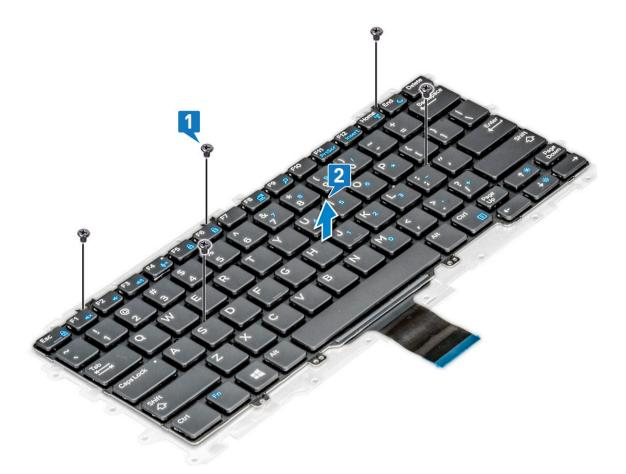
(i) NOTE: Remove the keyboard chassis when you encounter malfunction in the keyboard, after validating with a working laptop.
