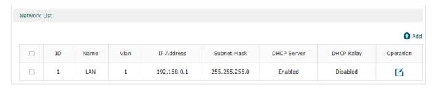
In the **Network List** section, set up the LAN network or click **Add** to add new networks, and configure the related parameters.
