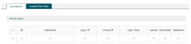
In the **Online Users** section, you can view the information of all the clients connected to the SSL VPN. You can also block or disconnect specific clients based on needs.
