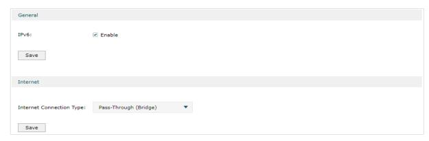
In **Internet** section, select the connection type as Pass-Through (Bridge). No configuration is required for this type of connection.
