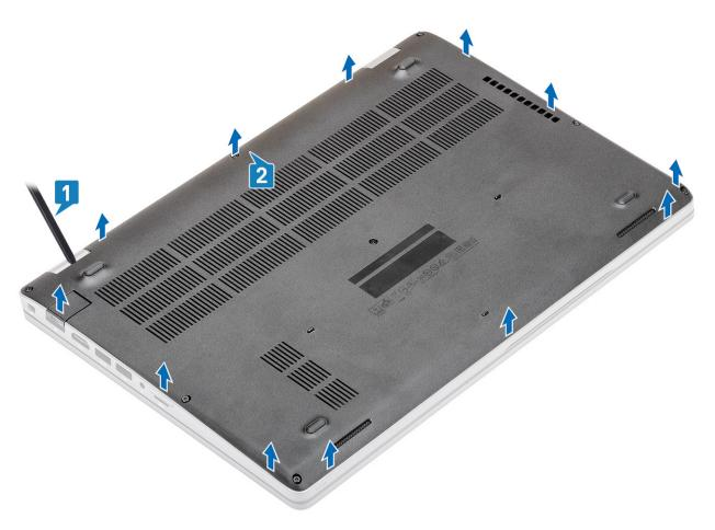
Lift and remove the base cover away from the computer.
