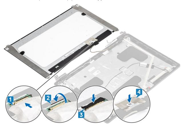
NOTE: LCD Panel comes with two (L+R) brackets that needs to toe-in first, then secure two screws located at the base of the LCD panel.
