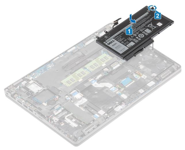
Connect the battery cable to the connector on the system board.
