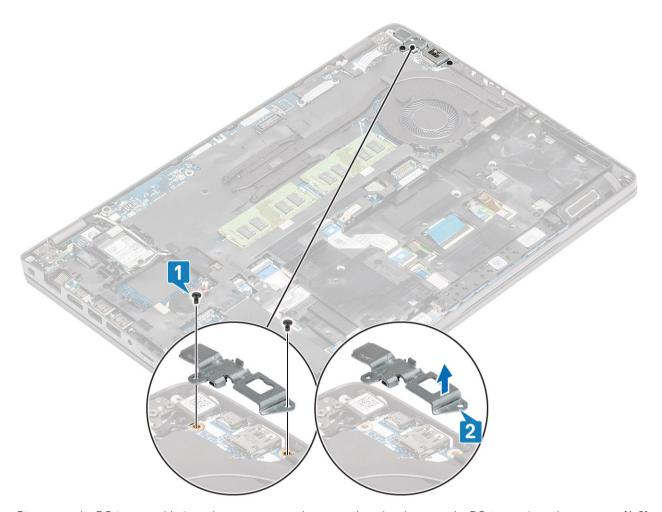
3 Disconnect the DC-in port cable from the connector on the system board and remove the DC-in port from the computer [1, 2].
