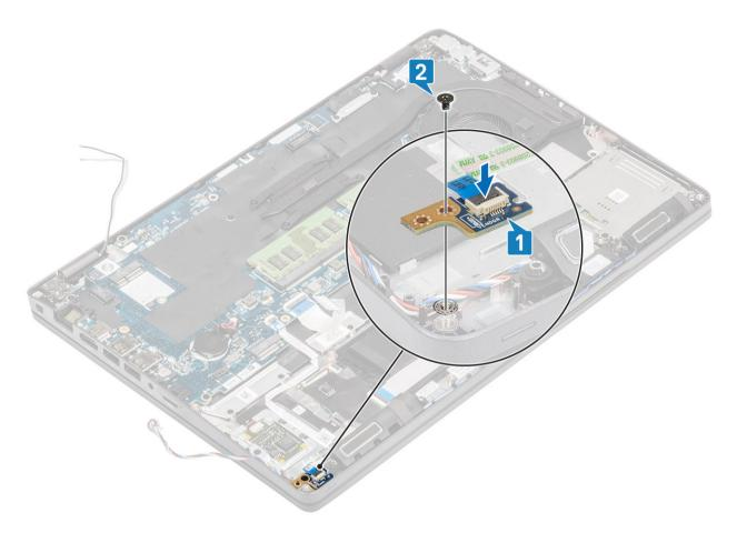
3 Connect the LED board cable to the connector on the system board and route the LED board cable [1, 2].
