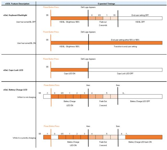
Power button with fingerprint reader will have no LED and will leverage the available LED's in the system to provide indication of the system status
