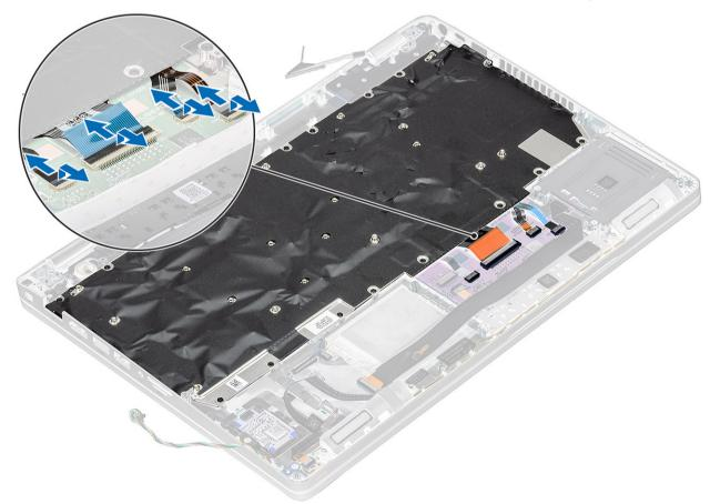
2 Remove the 22 (M2x2) screws that secure the keyboard to the palmrest [1].
