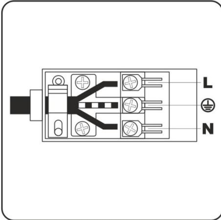
Correct grounding is a legal requirement. If the appliance is not pre-fitted with a power cable and/or plug, use only suitable cables and plugs capable of handling the power specified on the appliance's data plate and capable of resisting heat. The power cable should never reach a temperature 50 °C above ambient temperature at any point along its length.
