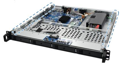
**b** Fasten the four screws you removed in step 2.
