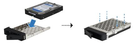
• For 2.5" drives: Place the drive in the drive tray. Turn the tray upside down and tighten screws into the four spots indicated below to secure the drive.
