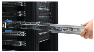
**5** Push the chassis towards the rack. Use the cage nuts and screws in the rail kit package to secure the chassis to the rack if necessary.
