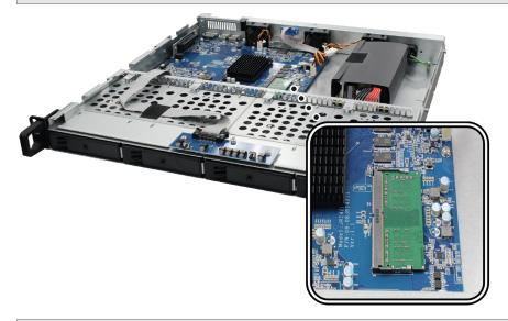
Important: RS820+ / RS820RP+ does not support ECC, regardless the expand memory being ECC or non-ECC.
