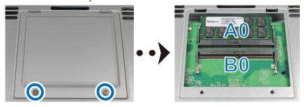
**Note:** When you remove the cover, sensitive internal components are exposed. Avoid touching anything other than the memory assembly when removing or adding memory.
