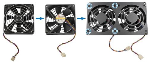
c Plug the fan cables into your Synology NAS as shown below.
