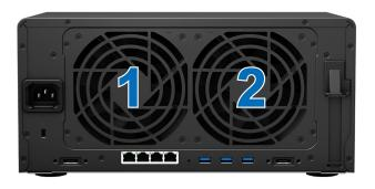
3 Remove the four screws that secure the fan panel.
