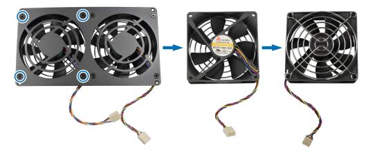
$\mbox{\bf d}$  Remove the screws that secure the fan guard from the malfunctioning fan.
