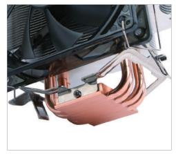
The 8mm thick copper coldplate and four copper heatpipes with Straight Touch technology quickly transfer heat away from your CPU
