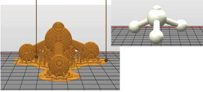
④ For models with non-manifold geometry (black-highlighted in the software), please repair the models before printing.
