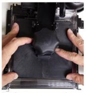
② Check if the tank is cloudy at where you place the model. Move the model away from the cloudy area in the software with the "Move" function. Replace the tank if the overall surface is cloudy.
