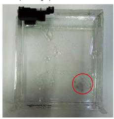
③ Brush the level sensor with alcohol if it gets stuck. Level sensor should return to the original position after a soft push. When the tank is full or the resin gets sticky, the sensor's movement may be hindered greatly. Normally, it may take 1 minute for sensor to return. If stuck, remove the remaining resin from tank before cleaning. If resin in tank is cured, please replace the tank.
