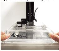
©Unpack the resin tank and insert it into the tank slot. Push all the way until reaching the end.
