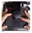
Place both hands over the platform to make sure the surface is adhered to the resin tanks. At the same time, tighten the fronts crews (F1, F2) with fingers and then the screws at the back (B1, B2). And then release both hands from the platform, fasten the 4 screws firmly.
