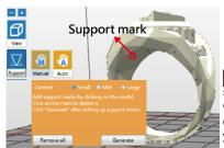
Manual editing: you may add or delete support structure based on the features of the print manually. To add support, simply select a proper size of the contact point and then click on the model at the overhangs. To delete support, just click on the support mark (the blue dot). After setting up support marks, click "Generate" to continue.
