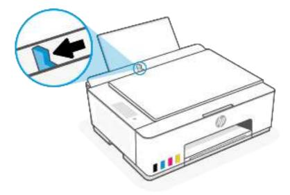
3. Insert paper into the input tray until it stops. Make sure paper is inserted in portrait orientation with the side to be printed facing up.
