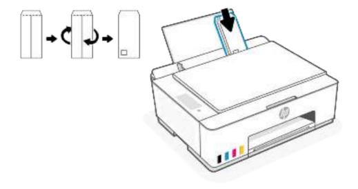
4. Slide the paper-width guide to the right against the stack of envelopes until it stops.
