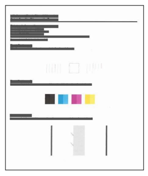
2. If the diagnostic page shows steaks or missing portions of the color and black boxes, then automatically clean the printheads.
