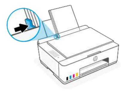
5. Pull out the output tray extender as shown.
