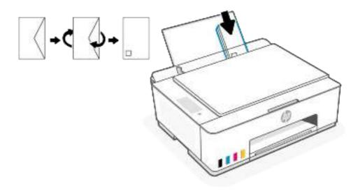
**b.** For envelopes with a flap on the short edge, insert vertically with the flap on top and facing down.
