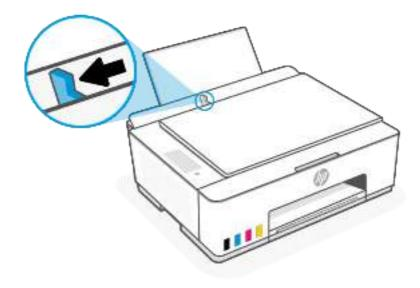
3. Insert one or more envelopes into the far-right side of the input tray, and slide the stack down until it stops.
