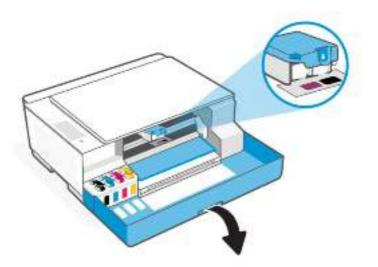
3. Press and release the blue latch to open the printhead cover.
