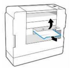
9. Close the bottom access door, making sure the two tabs click into place.
