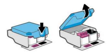
b. Remove the printhead from the carriage.
