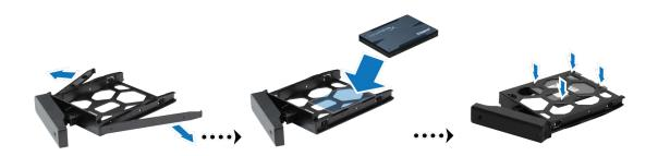
**4** Push the upper part of the loaded hard drive tray and insert it into the empty hard drive bay.
