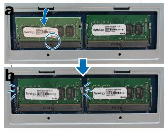
*Important:* You must utilize the same type of memory on all slots. The default memory is non-ECC SO-DIMM DDR4. If you expand utilizing ECC SO-DIMM DDR4 memory, you must remove the original.
