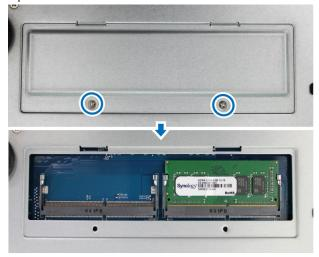
*Important:* When you remove the panel, you expose sensitive internal components. Avoid touching anything other than the memory assembly when you remove or add memory.
