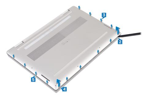
6 Move the base cover from left to right and lift the base cover from the palm-rest and keyboard assembly.
