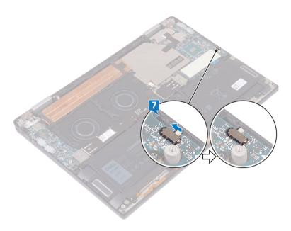
i NOTE: Turn-off the battery switch before you proceed to remove any other component from your computer.
