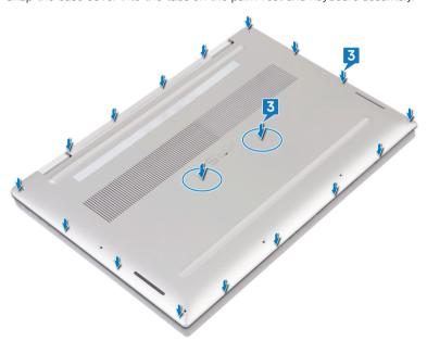
4 Replace the eight torx head screws (M2x3) that secure the base cover to the palm-rest and keyboard assembly.
