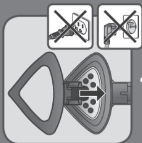
The crease attachment allows you to create a crease on your trousers or jackets. Attach the crease attachment to the steam head when appliance is unplugged and has cooled down.
