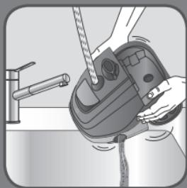
EN Vertically tilt the appliance to empty the water into the sink.
