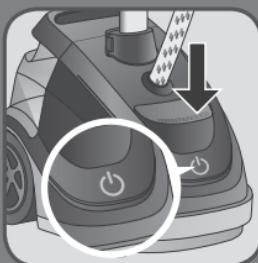
**EN** Press the On/Off Pedal and check that light is switched Off.
