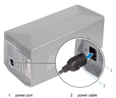
NOTE: It is recommended to shut down the computer and connect the Graphics cable from the Alienware Graphics Amplifier to your computer and then powering on the computer to dock with the graphics amplifier.
