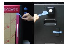
Insert the guide tube through the top cover, and then insert one end into the extruder module.
