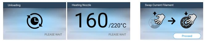
5. The nozzle will be preheated and the machine will notify you when to insert filament into the feed module.
