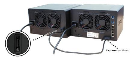
After the connection is complete, DX517 will be turned on or off automatically when the connected DiskStation powers on or off.
