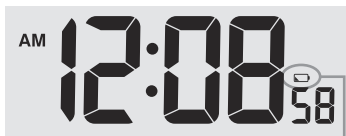
Low battery indicator for console
