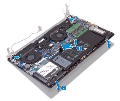
3 Using the alignment posts, press the hinges down on the system board and the palm rest and keyboard assembly.
