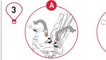
Connect the protective bars safety ring to the suitable left and right sides. Move them to the locked position adjacent to the steering bar and secure the mechanism. \_\_\_\_\_
