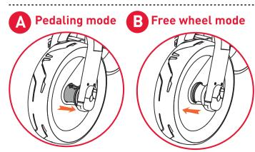
The pedals modes are interchangeable between FREE WHEEL and PEDALING MODES
