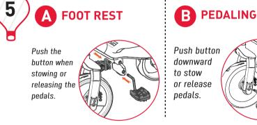
For toddlers aged 10-18 months it is recommended to set the pedals in FOOT REST mode and for 18 months and up to set the pedals in PEDALING MODE.
