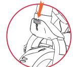
In order to change the steering mode the button must be lowered or raised accordingly while the steering bar and wheel are facing forward.
