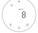
3 Touch and hold the 1 button for 3 seconds to switch off the air purifier.
