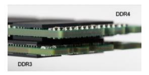
Figure 2. Thickness difference
