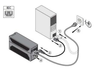
Connect the UPS to the AC-power source with cable through a wall outlet equipped with an earth connector, using your equipment cord.
