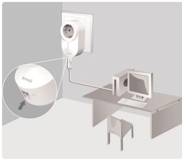
**Step 2** Connect the other adapter to a computer, and plug it to a wall receptacle nearby.
