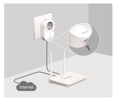
**Step 1** Connect one adapter to one of the LAN ports of a router for internet access, and plug it into a wall receptacle nearby.
