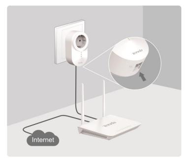
**Step 1** Connect one adapter to one of the LAN ports of the router for internet access, and plug it to a wall receptacle nearby.
