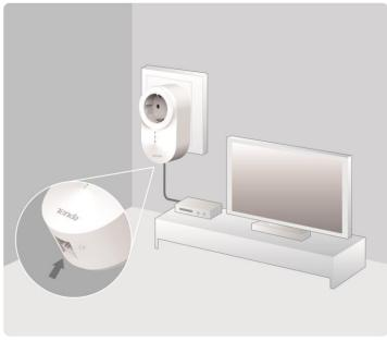
Step 2 Connect the other adapter to a set-top box of a TV, and plug it to a wall receptacle nearby.
