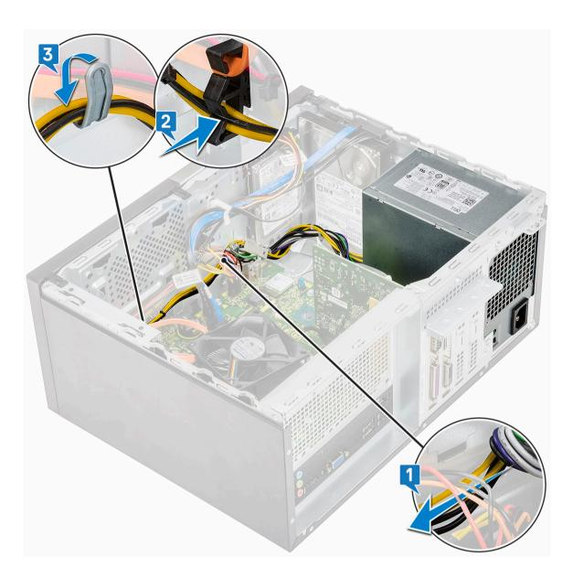
Connect the PSU cables to the connectors on the system board.
