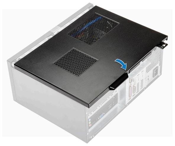
2 Tighten the two (6-32x6.35) screws to secure the cover to the computer.
