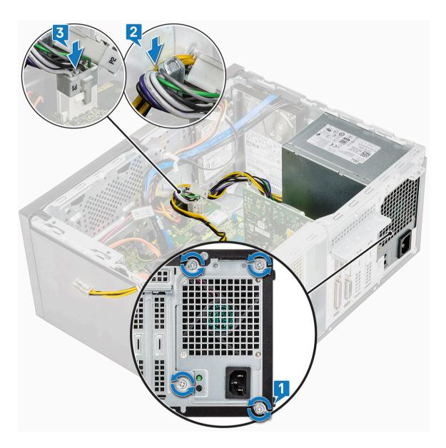
3 Route the PSU cables through the retention tabs.
