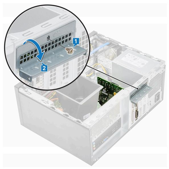
b Push the release tab [1] and lift the PCle expansion card out of the computer [2].
