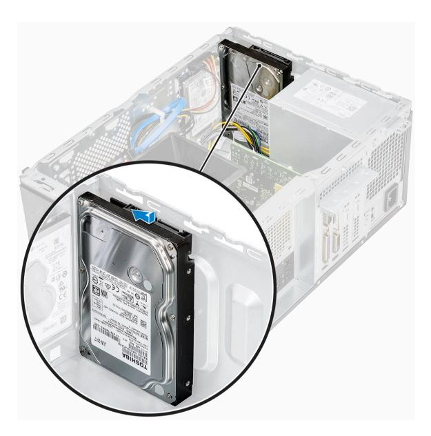
2 Install the four (6-32x3.6) screws that secure the hard drive assembly to the base and front of the chassis.
