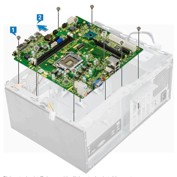
b Tilt the system board at 45-degrees, and then lift the system board out of the computer.
