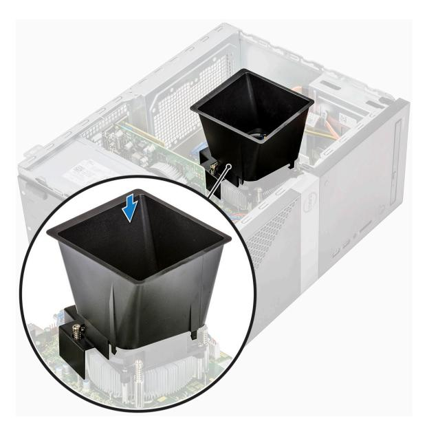
2 Lower the cooling shroud into the chassis and press down on the shroud until it snaps into place.
