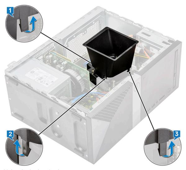
b Lift the cooling shroud away from the computer.
