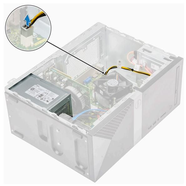
b Unroute the PSU cables from the retention clips.
