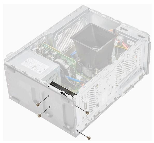
c Slide and lift the HDD away from the chassis
