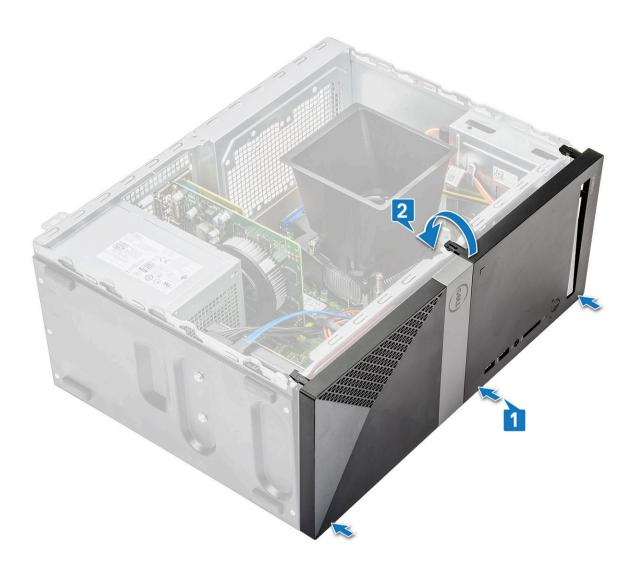
2 Rotate the bezel until the tabs clicks into place.
