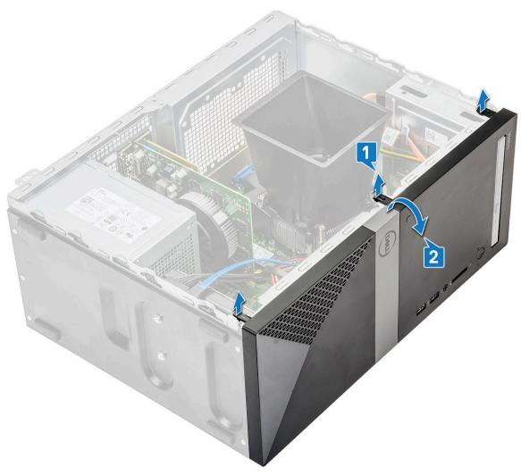
c Lift the chassis and remove the front bezel from the chassis
