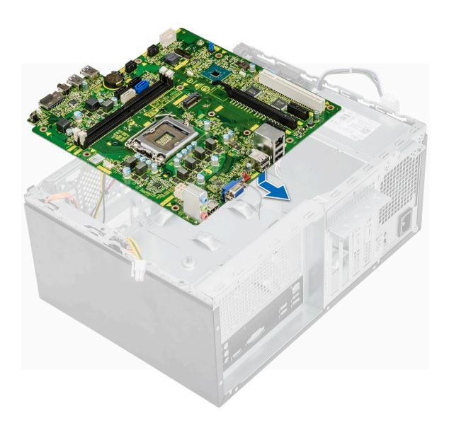
2 Tighten the eight (6-32x6.35) screws and one (6-32x4.8) screw for M2.SSD that secures the system board to the chassis.
