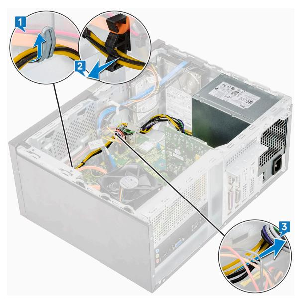
c Unroute the PSU cable from the metal clip [1], press the tab of the 8-pin power cables and disconnect it from the system board [2], and then remove 4 (6-32x6.35) screws to release the PSU [3].
