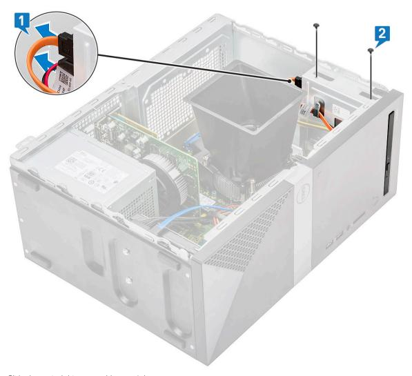
c Slide the optical drive assembly out of the computer.
