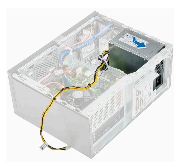
Tighten the four (6-32x6.35) screws to secure the PSU to the computer [1], route the PSU cable from the metal clip [2] and insert the 8-pin power cables [3].
