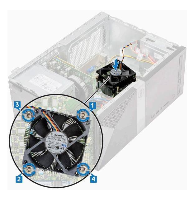
3 Connect the fan cable to the connector on the system board.
