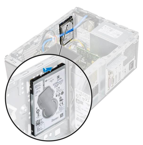
2 Install the two (M3x3.5) screws that secure the hard drive assembly to the base and front of the chassis.
