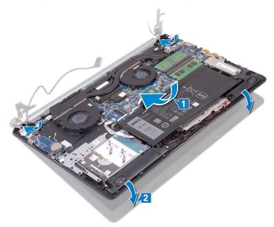
3 Using the alignment posts, press the hinges down on the system board and the palm rest and keyboard assembly.
