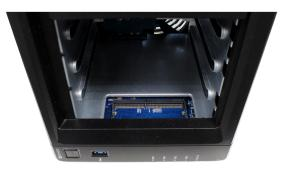
**Note:** When you remove the drive trays, sensitive internal components are exposed. Avoid touching anything other than the memory assembly when removing or adding memory.
