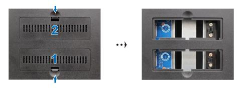
Note: Hold the SSD module by its edge and avoid touching the gold connectors.
