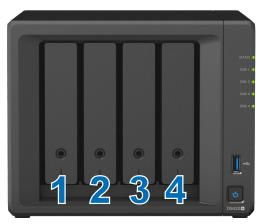
**Note:** If you plan to create a RAID volume, we recommend installing drives of identical size to make the best use of drive capacity.
