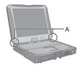
Use the tether to attach the stylus to the computer so you will not lose it. There are holes (A) to attach it.
