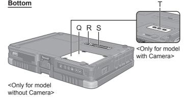
Insert the SIM card into the SIM Card Slot with the contact side facing downward and with the cut corner oriented as shown in the illustration.
