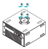
Attach the other VESA Bracket to the rear of a compatible display using the four screws.
