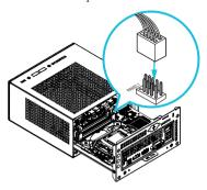
2. Align the motherboard tray with the two sliding tracks on the chassis while sliding it back to the chassis.
