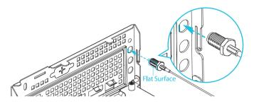
2. Fasten the screw nuts to secure the antenna connectors.
