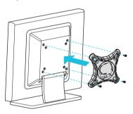
3. Mount the DeskMini 310 series by turning it counterclockwise.
