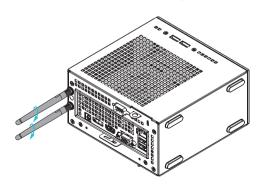
4. Set the WiFi 2.4/5 GHz Antenna at 90-degree angle.
