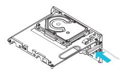
6. Connect the other end of the SATA Cables to the SATA Connectors on the motherboard.
