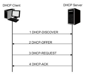
Figure 5-18 Interaction between a DHCP client and a DHCP server
