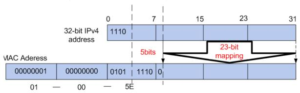
Figure 8-2 Mapping relationship between multicast IP address and multicast MAC address
