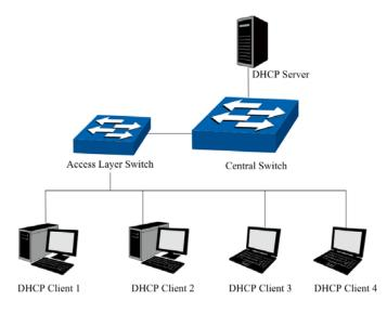
Figure 5-17 Network diagram of DHCP
