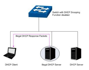
Figure 5-19 DHCP Cheating Attack Implementation Procedure
