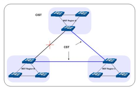
Figure 7-2 Basic MSTP diagram
