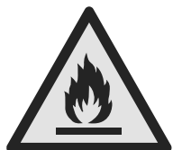
Caution: Risk of fire/ flammable materials
