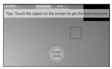
4) Tap Start Scan, the object would automatically rotate on the turntable, and a 3D model will display after the scan finishes;
